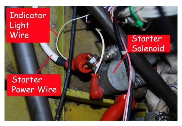
Figure 5 Starter Solenoid Wiring
