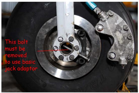
Figure 4. Axle Retainer Bolt To Be Removed
