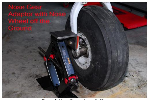
Figure 2. Nose Gear Adaptor In Use
