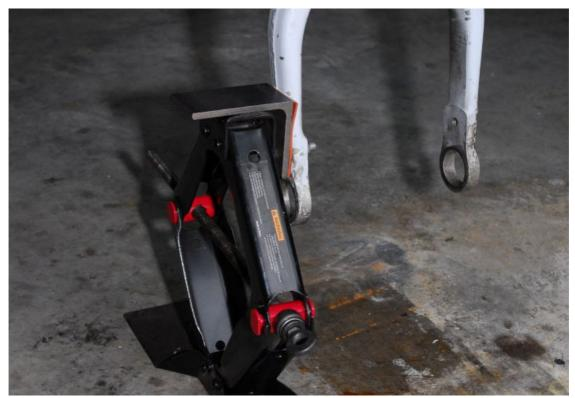
Figure 3. Nose Gear Adaptor With Wheel Removed
