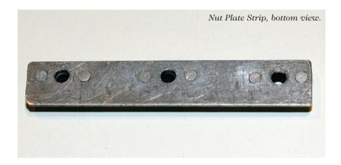
screw grip from bottoming out. Because I used nut plates, I couldn't use washers, and it was much easier to use full thread screws of adequate length. This did not present a problem, however, since the screws themselves are not used specifically to line up the structures through which they pass, but rather to hold the hinge in place by sandwiching it between two layers of aluminum sheet. Thus there is no need to have a grip on the screws.
