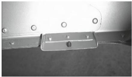
Plate, main gear door stop repair showing added doubler
