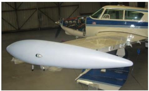
The tip tank laid up on one of the wings
