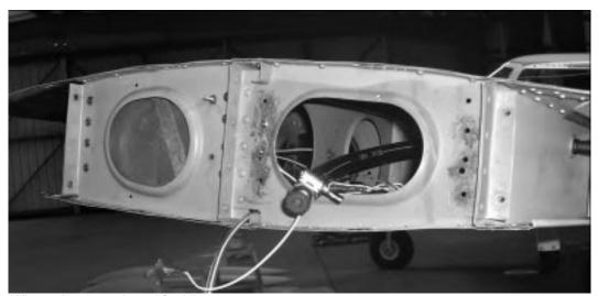
Where the tip tank and fuel line connect
