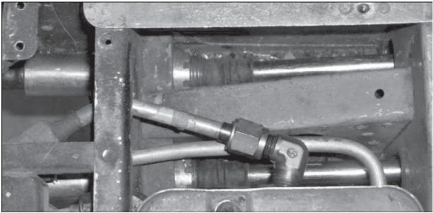
The new conduits routed through the under-seat bulkhead.
