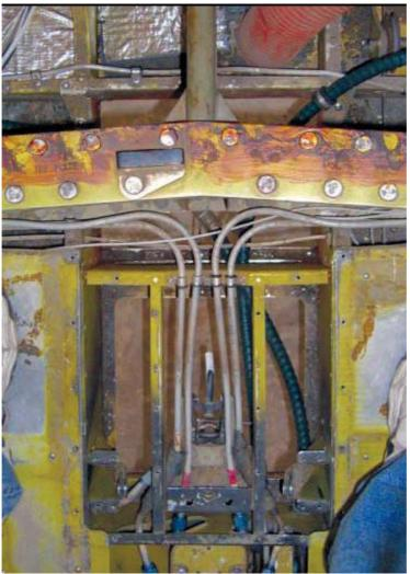
A top-view look at the new conduits installed and routed.
