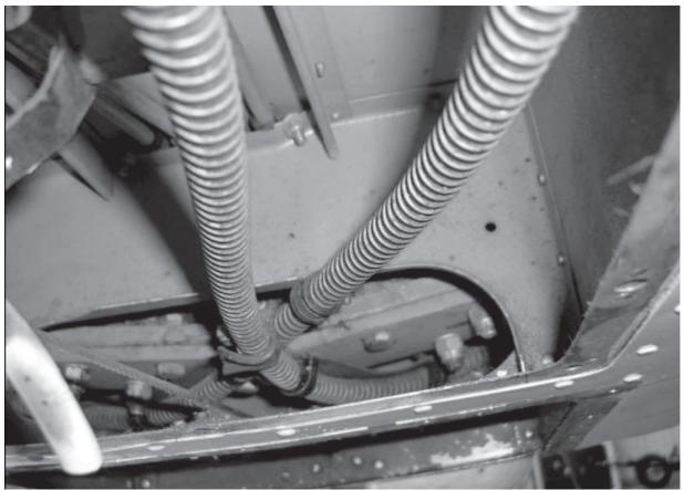
Looking aft at the old conduit routing, the left conduit goes under the right one.
