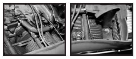
Figure 3 (left): Short fuel line with 45-degree adaptor and bulkhead union. Figure 4 (right): Hole plug in shroud.
