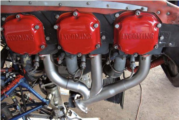
Dual exhaust, right-side manifold installed.
