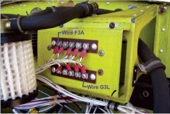
Figure 1: Flasher Box Assembly, F3A and G3L denote wire markings.
