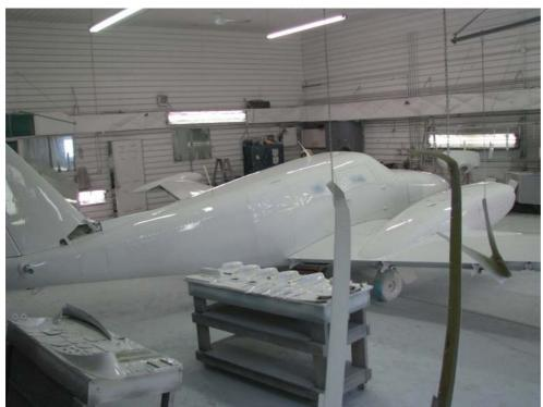
The first layer of paint with some of the 100 removed parts.
